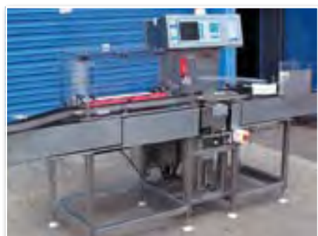
4E 2848 GRASEBY BEST model D30 inline checkweigher
