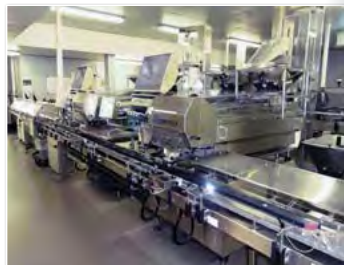
1A 3094 SWIFTPACK high speed tablet counting line
