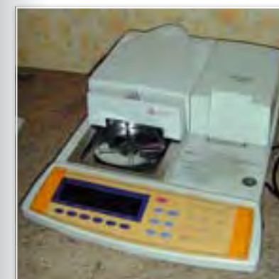
9 2292 SARTORIUS model MA 50 moisture analyzer
