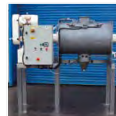
7C 2946 MORTON 300 Litre stainless steel ploughshare mixer
