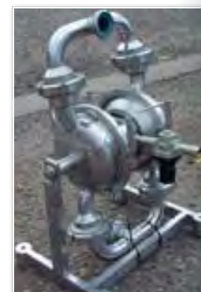
8C 2517 DEPA model DL40 SL hygienic double diaphragm pump
