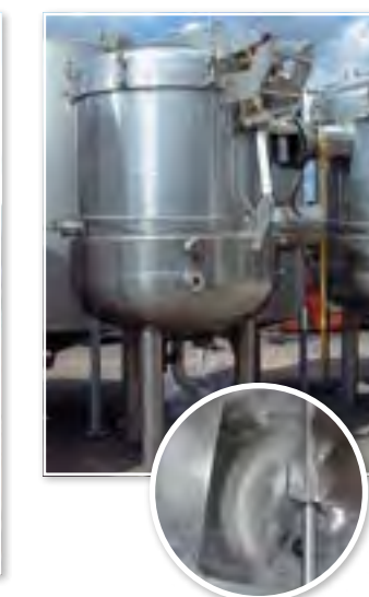
2A 1880 1500 litre BCH scraped surface over-mix vessel
