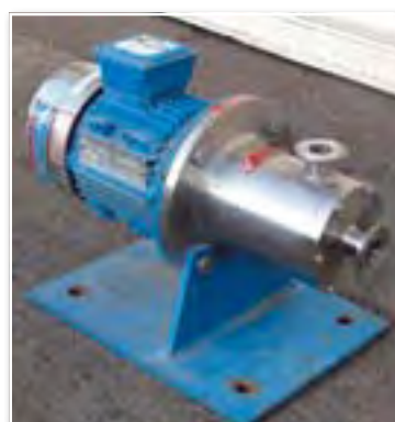
5B 3208 SILVERSON type 200L inline homogeniser
