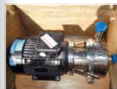
3270 MIDLAND DAIRY model D3/4K centrifugal pump
