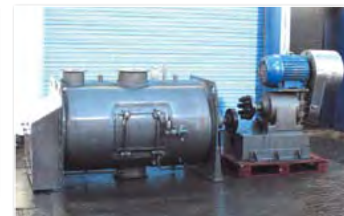
7C 2948 MORTON 1000 litre stainless steel ploughshare mixer
