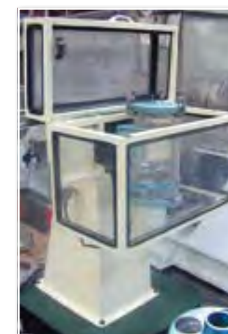
5A 2671 TP ENGINEERING type 755 powder blender
