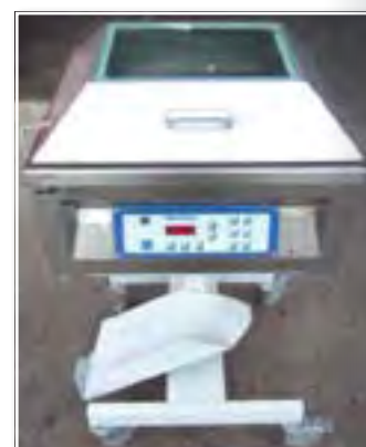
4D 3277 MULTIVAC bag sealer type A300/16
