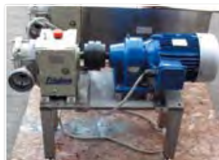
8B 3101 FRISTAM FLK25 S/S claw type pump
