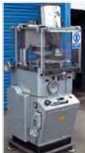
1A 2912 KILIAN model RTS, 20 station tablet press
