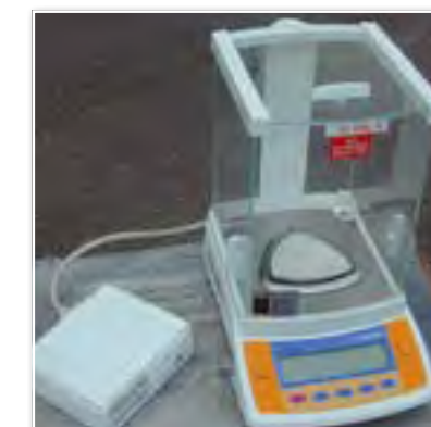
2716 SARTORIUS type CP225D-0EC lab weigh scale
