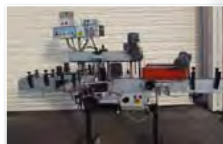
4A 3139 ATTWELL type "Molly" 2500 front & back labeller
