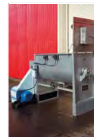
5A 3191 ARENCO ALITE type 24/2 single spiral S/S ribbon blender
